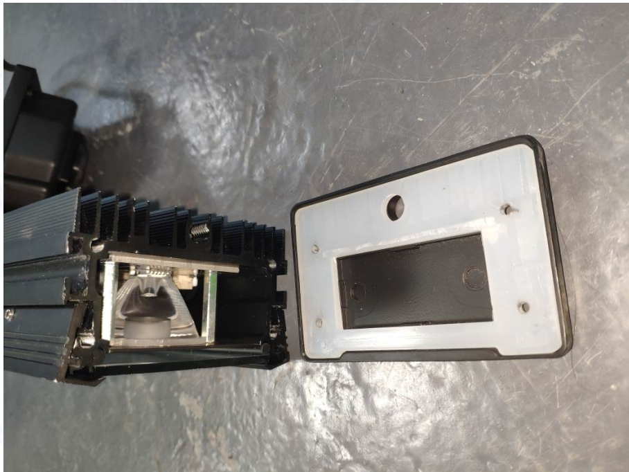
Photo 6: after Jet-proof test view
