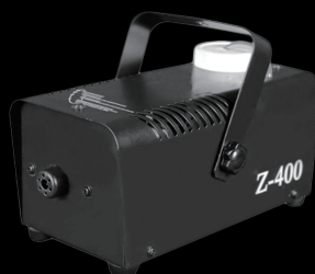
Z-400 • Voltage: 100-240V AC 50/60HZ • Power Consumption: 400W • Controller Mode: Wired control • Tank Capacity: 0.3L • Coverage: 2000cu/ft/min • Spraying Distance: 1.5~3.5m
